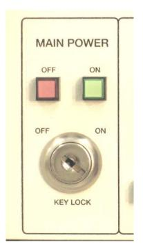
The Main Power has a Key Lock Switch that prevents unauthorized access to the Power Supply. The OFF button lights red after the Key Lock Switch is turned on. The ON push button lights green when the main power is on. If the Key Lock is turned off, no lights will be lit. Before you turn on the main power, make sure that you have turned on the Magnetic Hydraulic Circuit Breakers located on the Front Panel of the Power Module.
