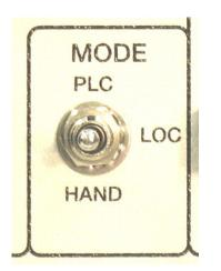
The Control Source Switch, located below the power meter, has three settings to select the source from which the High Voltage and Emission Current will be controlled.
